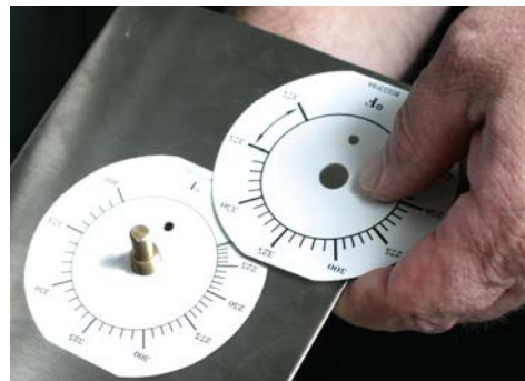
Figure 7: The faceplate on the potentiometer must be replaced. Align the new one with the holes on the existing faceplate.
