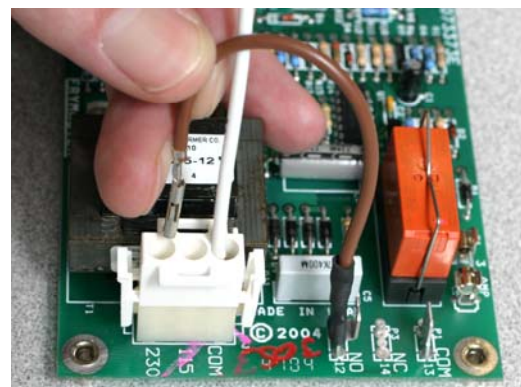
Figure 2: Plug the brown wire into the appropriate power outlet on the plug, 115 or 230.
